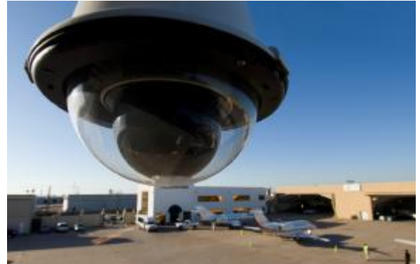
Pan/tilt/zoom camera viewing Million Air's FBO and ramp area.
